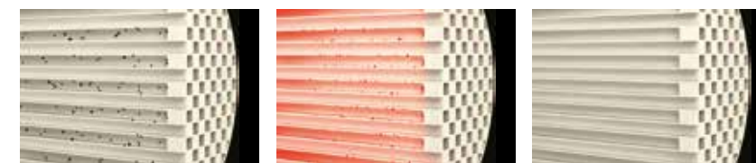
1. Particulate matter trapped 2. Regeneration starts 3. Regeneration completes*
